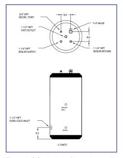
Figure 2: C Series Unit - Dimensions and Connections
