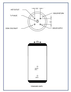
Figure 1: Standard Unit - Dimensions and Connections
