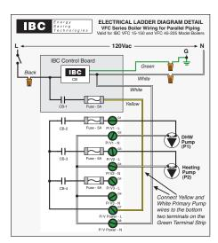
On a VFC Model boiler, locate the Yellow and White pair of wires in the wiring box behind the IBC Control. Connect the Yellow wire to the "P/V Power L" terminal second from the bottom on the Green terminal plug. Connect the White wire to the bottom terminal labelled "P/V Power N". This will satisfy the boiler's flow proving routine when either zone starts up.
